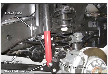
MARNING: Do not allow the front axle to hang by any hoses or cables. You could damage the hose or cable, without this damage being visible to you, resulting in sudden and unexpected failure and an accident.
