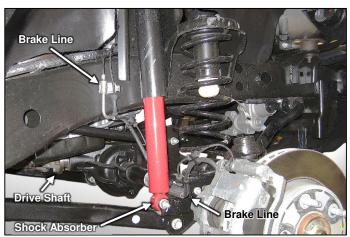
⚠ WARNING: Do not allow the front axle to hang by any hoses or cables. You could damage the hose or cable, without this damage being visible to you, resulting in sudden and unexpected failure and an accident.
